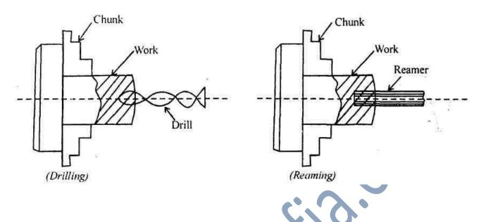
(v) **Reaming** : It is an operation of finishing the previously drilled hole. In the operation as shown in fig., a reamer is held in the tailstock and it is fed into the hole in the similar way as for drilling.
